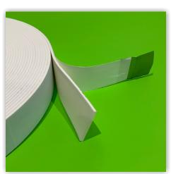
Manufactured from a hard white predominantly closed-cell impact foam and a pressure sensitive acrylic adhesive, this specialist tape creates a water, air and dust seal when compressed. It is ideal for cushioning or gap filling and provides a vibration and rattle-free seal between structural steel and panelling systems or the support brackets for pipework, cabling and HVAC trunking.
